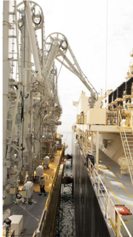
A tanker being loaded with LNG at ExxonMobil's terminal in Papua New Guinea.
