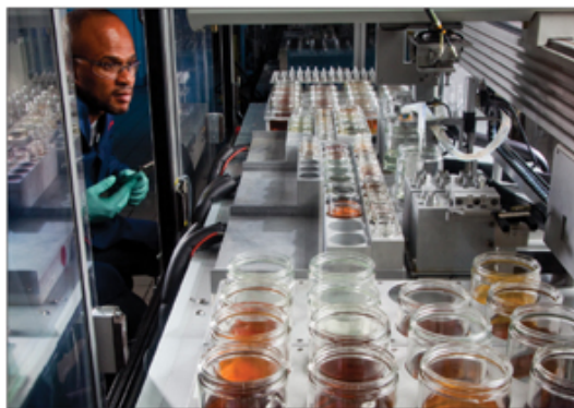
High-throughput research equipment, like this automated lubricant blending station, enables our formulators to rapidly map results from component modifications to deliver improved product performance.
