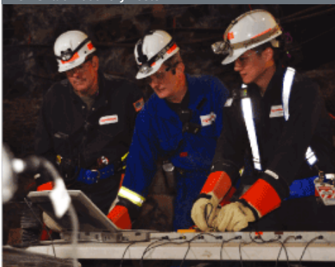
Researchers measure voltages in an Electrofrac oil shale heating experiment at ExxonMobil’s Colony Mine in Colorado.
