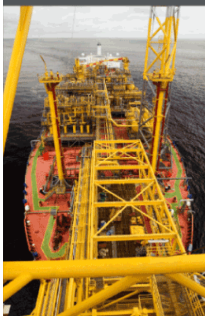
The Kizomba C Mondo project uses a floating production, storage, and offloading (FPSO) vessel that was converted from a tanker.
