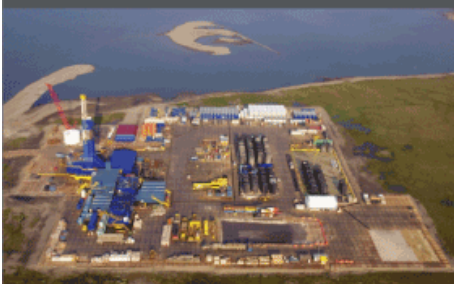
On Alaska's North Slope, development drilling has commenced at the Point Thomson Unit. The operation is being supported by barge in summer and an ice road in winter.
