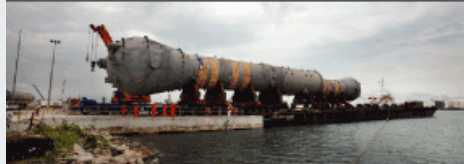
(Left) The expansion of the Singapore complex includes world-scale polyethylene reactors. (Below) Polyethylene reactors being taken off of barges upon their arrival in Singapore.
