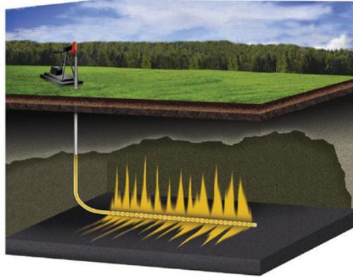
In Cyclic Solvent Process (CSP), solvent (yellow) is injected through a horizontal wellbore into the reservoir to reduce the viscosity of heavy oil in place. After injection, a solvent-oil mixture is produced through the same wellbore.
