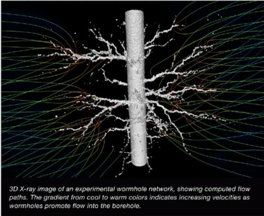
3D X-ray image of an experimental wormhole network, showing computed flow paths. The gradient from cool to warm colors indicates increasing velocities as wormholes promote flow into the borehole.
