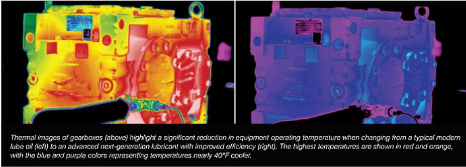
Thermal images of gearboxes (above) highlight a significant reduction in equipment operating temperature when changing from a typical modern lube oil (left) to an advanced next-generation lubricant with improved efficiency (right). The highest temperatures are shown in red and orange, with the blue and purple colors representing temperatures nearly 40°F cooler.
