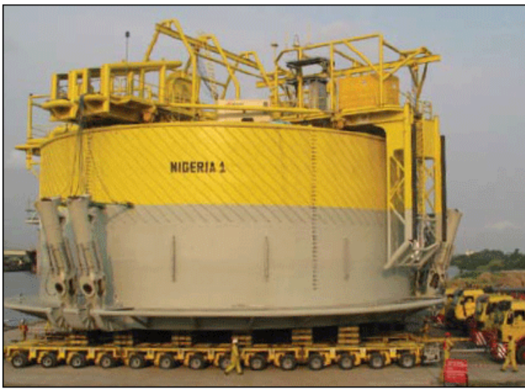
The Erha field's offshore loading buoy, one of the largest in the world, was fabricated in Lagos, Nigeria.
