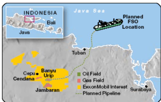
(Above) Appraisal drilling in preparation for development of the Banyu Urip field began in 2007. (Below) As planned, the Banyu Urip development consists of about 50 wells, a 20-thousand-barrels-of-oil-per-day early production facility, an onshore central processing facility capable of handling 165 thousand barrels per day, and a 60-mile pipeline that connects to a 2-million-barrel floating storage and offloading vessel (FSO).
