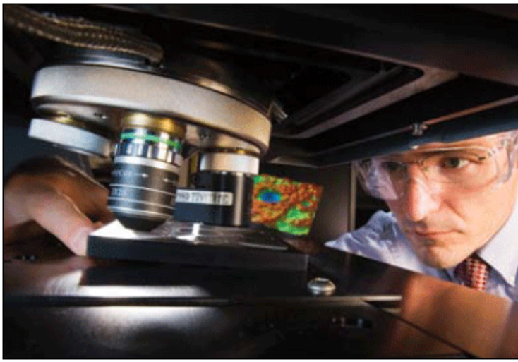
ExxonMobil scientists analyze corrosion using an interferometric microscope.
