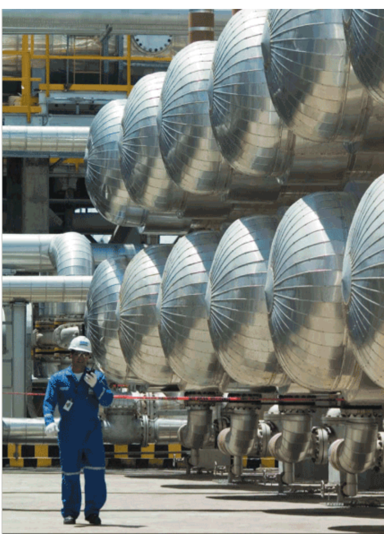
Diluted crude oil is treated at the Cerro Negro central processing facility, Venezuela, to remove associated gas, water, and salt. The crude is then transported approximately 185 miles to the Cerro Negro Upgrader for upgrading to a synthetic crude oil before shipping to the Chalmette refinery in the United States.
