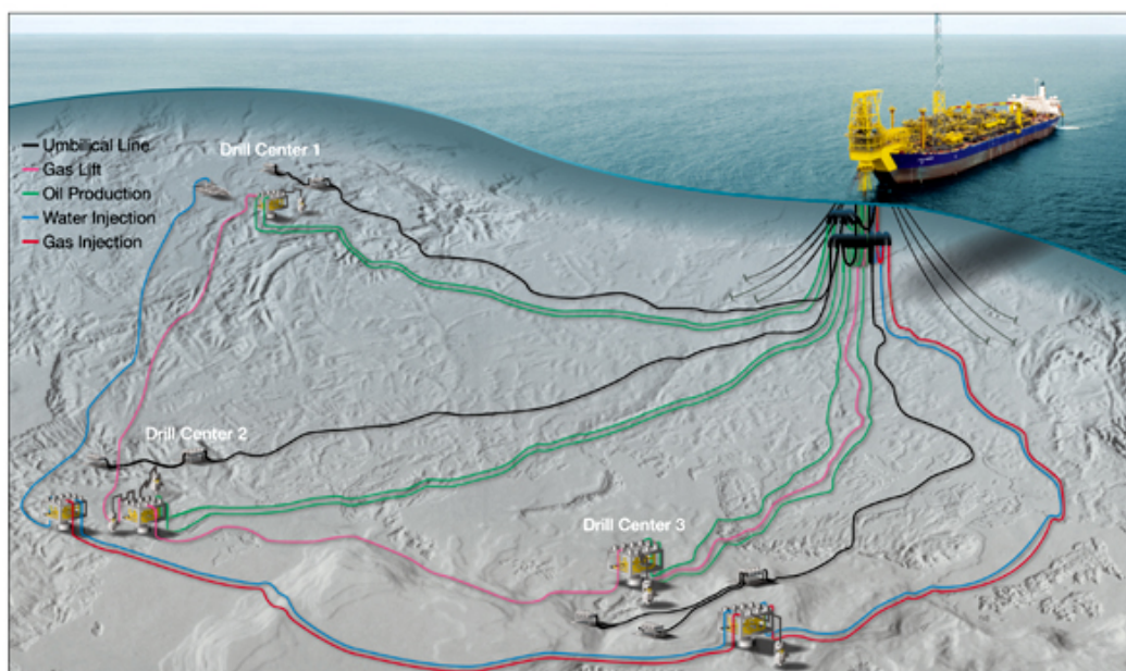
The Kizomba C Mondo project is a subsea tieback of three drill centers to a floating production, storage, and offloading (FPSO) vessel with a capacity of 100 thousand barrels of oil per day.
